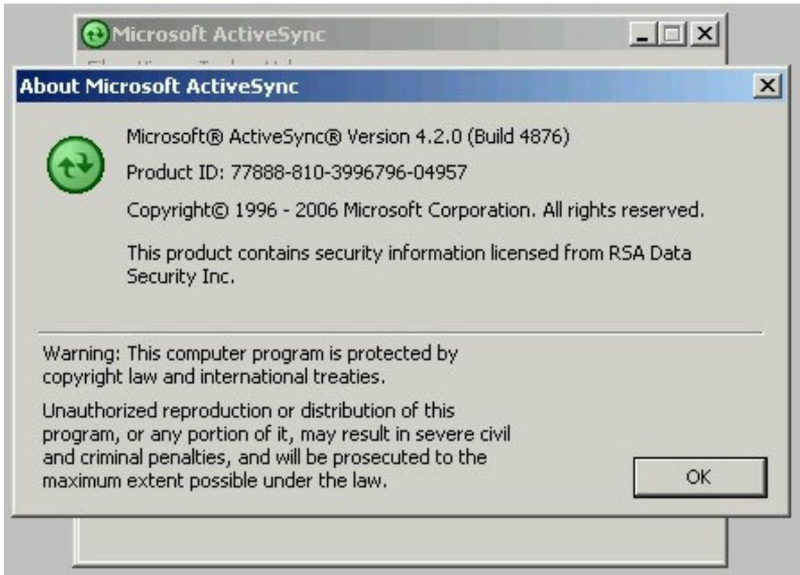
Making the connection to ActiveSync is as simple as connecting the USB cable from the MobileMapper CE I/O module to the PC. Once the hardware connection is made ActiveSync will find the MobileMapper CE and ask what you want to do.
